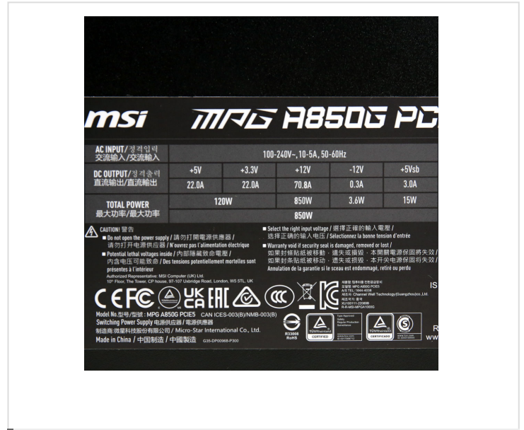
Power specifications label
