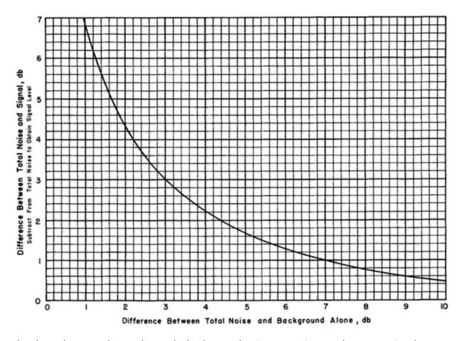
The chart above can be used to make background noise corrections to the source signal.
