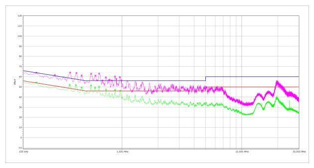
These are the results of a PSU failing both the average and quasi-peak detectors. Both have to be a "pass" for the PSU to meet the CISPR 32 / EN55032 requirements.
