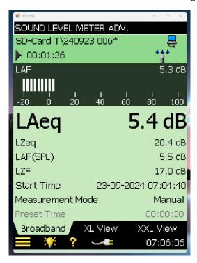
In no case can the background noise exceed the sound of interest, and in practice, the output level of the DUT has to be at least 3 dBA higher than the background noise for the measurement to be accurate. Still, a correction has to be applied to get the correct result. The background noise correction is defined as K1 [9] [11], and it is the amount the measured source level is reduced to obtain the background noise-corrected source level.
