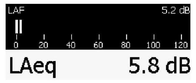
The noise measurements are conducted with Class 1 Bruel & Kjaer sound analyzers (2270 G4 and 2250-L G), equipped with type 4955-A low-noise and free-field microphones, which can measure down to 5 dB(A) (we also have type 4189 microphones that features a 16.6-140 dBA-weighted dynamic range). The sound analyzers are installed into a hemi-anechoic chamber, with a close to 6 dB(A) noise floor. A Bruel & Kjaer Type 4231 is used before every noise measurement to calibrate the sound analyzers.
