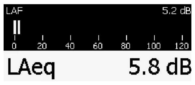
The noise measurements are conducted with Class 1 Bruel & Kjaer sound analyzers (2270 G4 and 2250-L G), equipped with type 4955-A low-noise and free-field microphones, which can measure down to 5 dB(A) (we also have type 4189 microphones that features a 16.6-140 dBA-weighted dynamic range). The sound analyzers are installed into a hemi-anechoic chamber, with a close to 6 dB(A) noise floor. A Bruel & Kjaer Type 4231 is used before every noise measurement to calibrate the sound analyzers.
