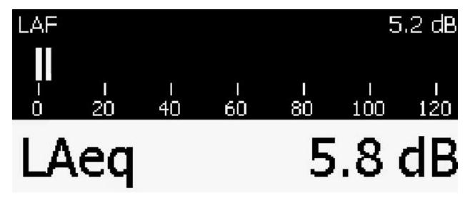
The noise measurements are conducted with Class 1 Bruel & Kjaer sound analyzers (2270 G4 and 2250-L G), equipped with a type 4955-A low-noise and free-field microphones, which can measure down to 5 dB(A) (we also have type 4189 microphones that features a 16.6-140 dBA-weighted dynamic range). The sound analyzers are installed into a hemi-anechoic chamber, with a close to 6 dB(A) noise floor. A Bruel & Kjaer Type 4231 is used before every noise measurement to calibrate the sound analyzers.
